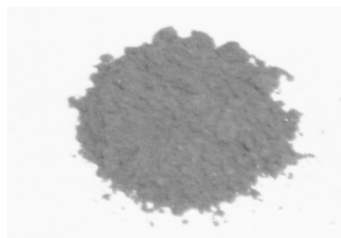
Place 3a, 58.7%Al, 69w% of all deposit (test type G at 1515°C)
